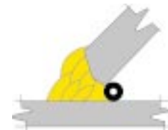
5 Connection between angled side wall and tank floor
