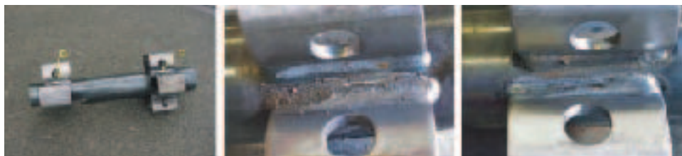
Figures 12a,12b,12c. Another component (12a) welded with solid wire (12b) and with PZ6105R (12c).
