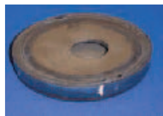
Figure 2. Safety component welded with PZ6105R
